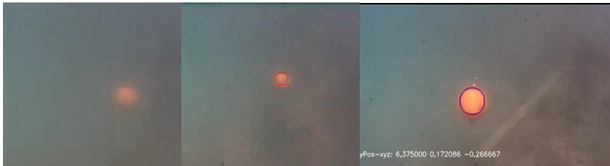
Figure 4b: SAUC-E 2011 Bremen's buoy servoing: detection, initial lock on it, final tracking and circling around it.
